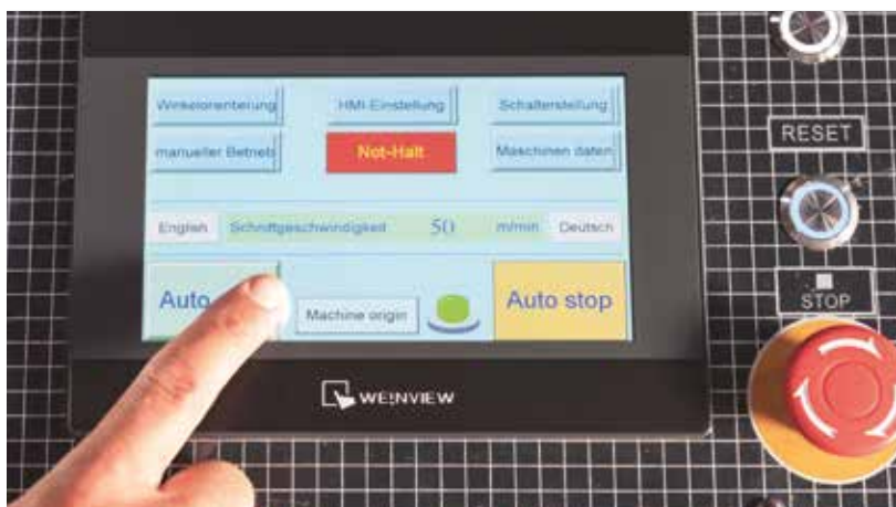
In Auto Mode, feed distance, cut angle, and number of cuts can be programmed within the respective configurations
