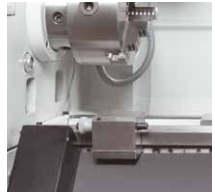
Micrometer bed stop ensures repeatability
