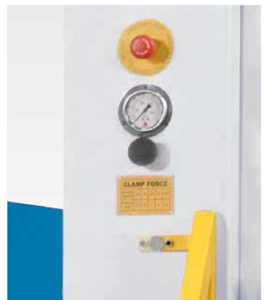
Adjustable upper die clamping pressure
