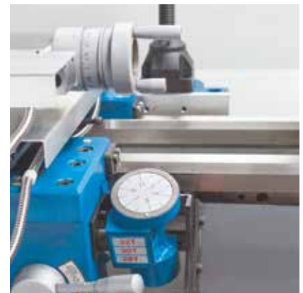
The thread gauge allows for resuming the thread after the apron nut for retrograde motion has been opened
