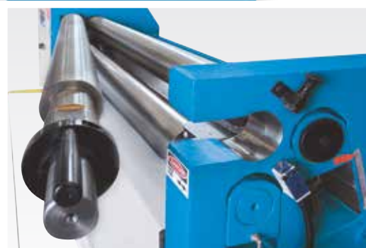
Upper roller can be swiveled out
