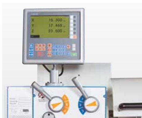
Positioning indicator on X-, Z- and Z1-axis
