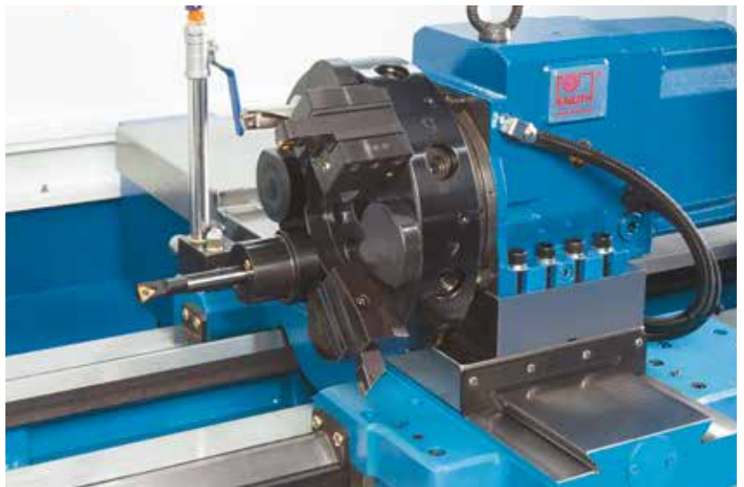
VDI 30 Tool Turret with 8 stations (Numturn 420 SI)
