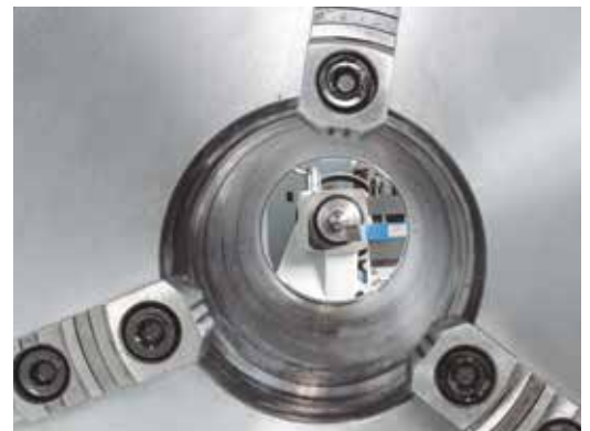
Spindle bores up to 225 mm
