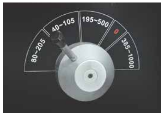
4 gear stages for high torque in the entire speed range
