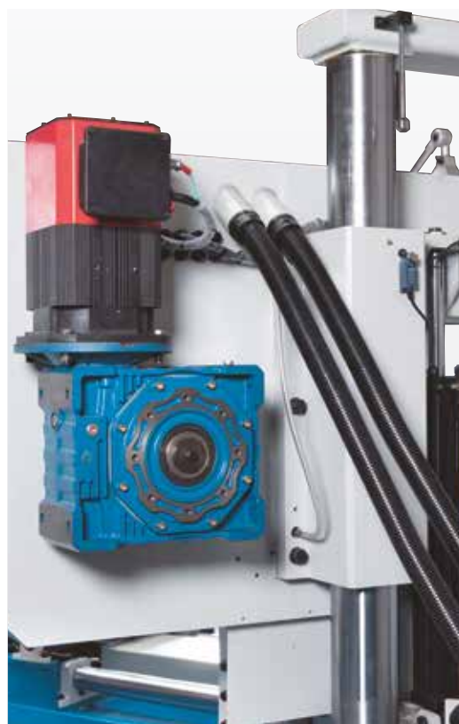
Infinitely variable high-torque servo-motor
