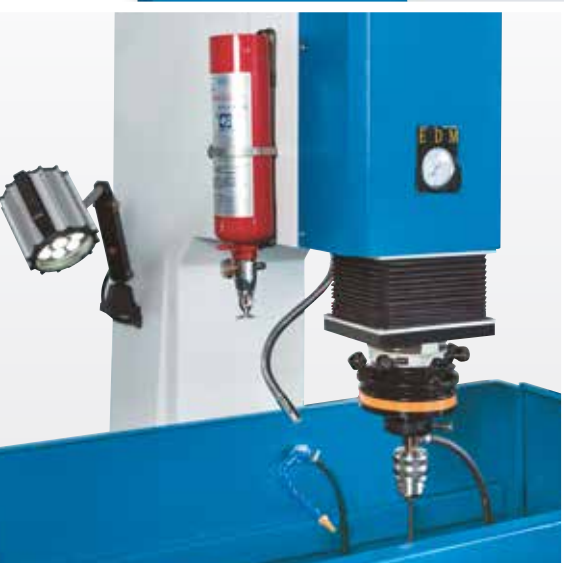
Fire extinguishing system for added safety
