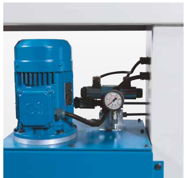
Compact hydraulic unit for powerful tube clamping
