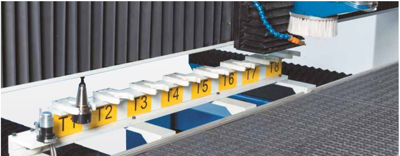
Linear 8-station tool changer
