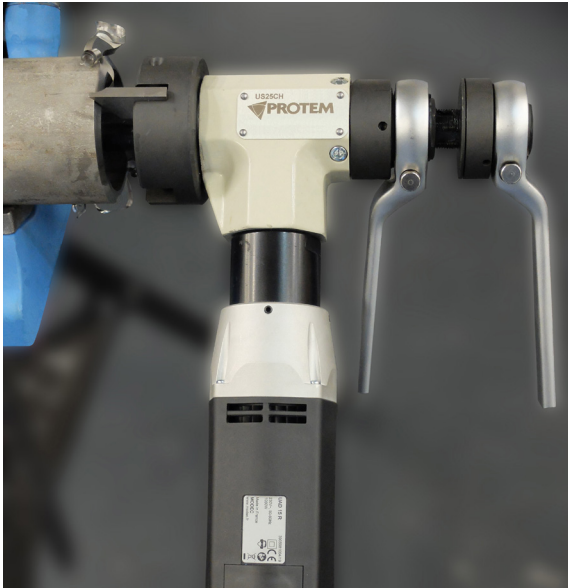
US25CH with pneumatic drive
