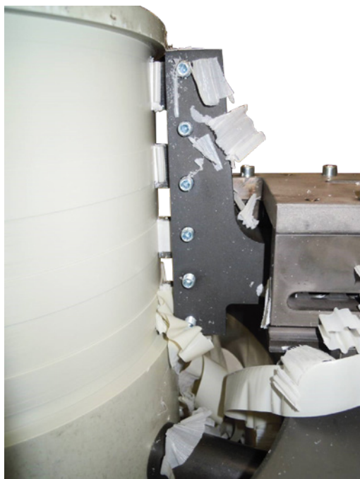
PROTEM TTNG-HD Orbital cutting machine with coating removal option
