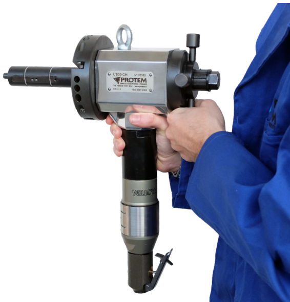
US30CH with pneumatic drive
