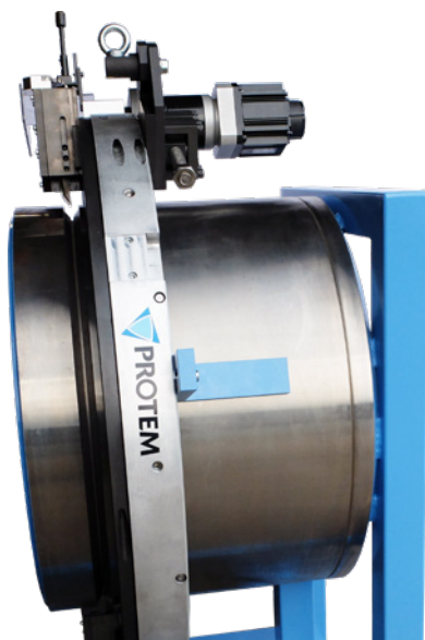
Protém TTNG-HD orbital cutting machine with Brushless Motor
