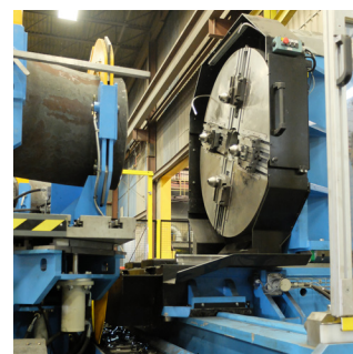
Elbow Beveling Machine
