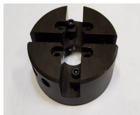
Tool-holder Plate 90mm
