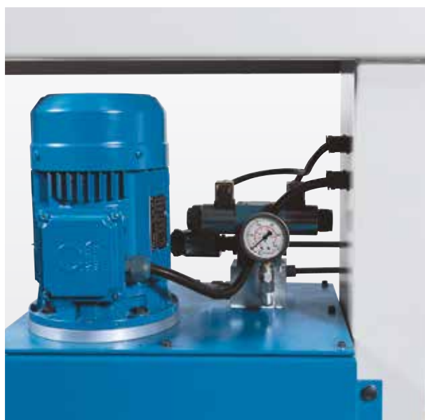
Compact hydraulic unit for powerful tube clamping
