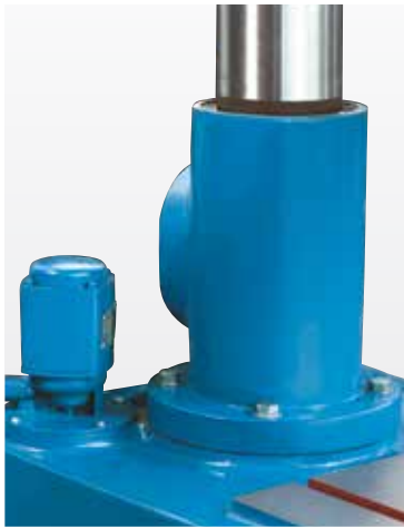
Coolant system is integrated into the machine base (KSS 25V, KSS 32)
