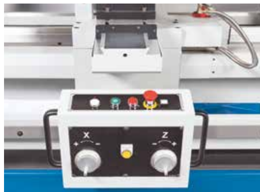
Compact control unit with electronic hand-wheels
