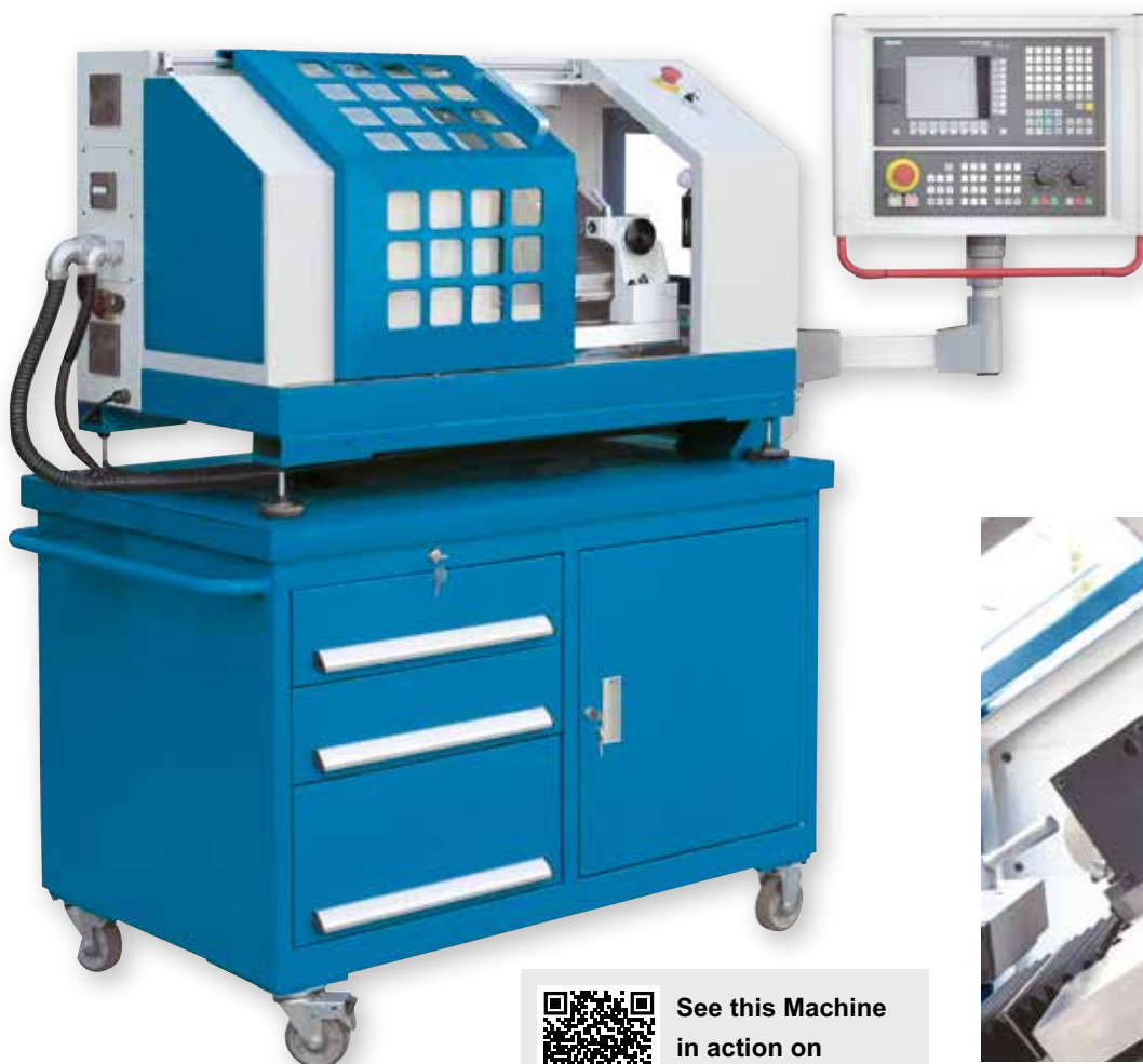
Inclined bed design optimizes work space and chip removal
